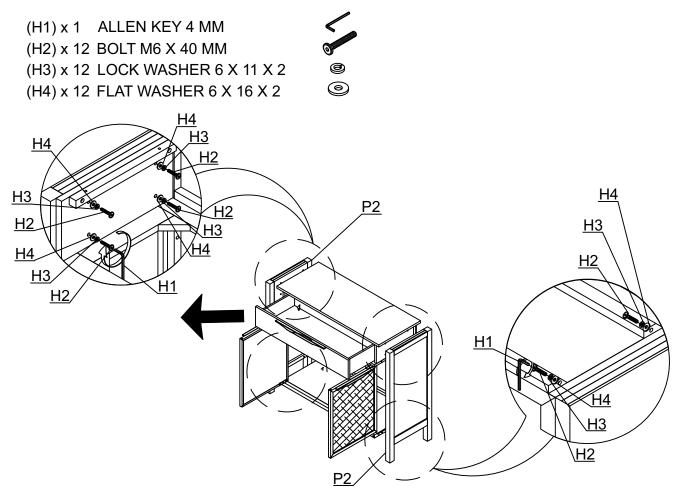
Step 4: Close the Drawer to main body, then tighten Side panel (P2) to Back panel (P3) using Allen key (H1), Lock Washer (H3), Flat washers (H4), and 40 MM Bolt (H2) as shown below.
